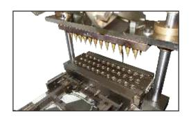
The ZE 25 series of semi-automatic machines are used for baking ice cream cones, moulded sugar cone and cups. These machines are easy to use and robust. The heating is by electrical heaters designed to optimize energy use and thermal distribution; This machine is flexible for high production on nonstop basis for 24 hours.
